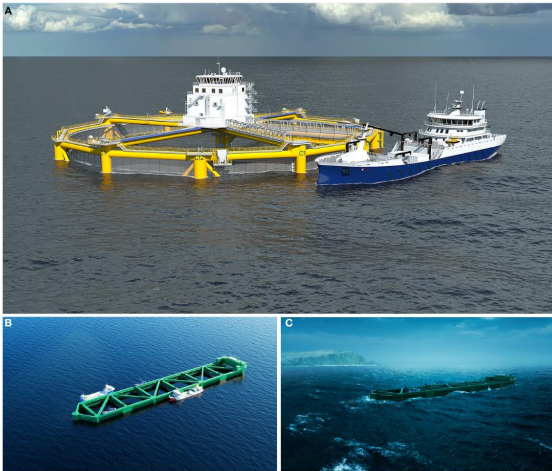
FIGURE 5 | (A) Large offshore fish farm device with a diameter of 110 m, a height of 67 m and a volume of 245,000 m 3 (upper image). This fish farm was just recently built in an Asian shipyard, transferred to Norway and could produce 6,000 t of salmon. (B,C) Havfarm 1 : Large aquaculture production unit integrated into a vessel-like floating platform in calm (B) and rough (C) conditions at sea (lower left). Havfarm 1 includes next to the large cages a mini-harbour for service vessels, maintenance trolleys along the outer rails providing access to the entire facility, rotatable thrusters to reduce stress on the mooring during storm conditions while also ensuring optimum oxygen supply, and a deep steel louse skirt, which reduces the risk of lice infection as well as protects the facility from being damaged by drifting objects [Image (A) with permission of NSK Ship Design and image (B) with permission of Ocean Farming AS].
